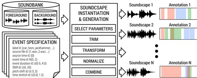
Figure 1: Block diagram of the Scaper synthesis pipeline.
