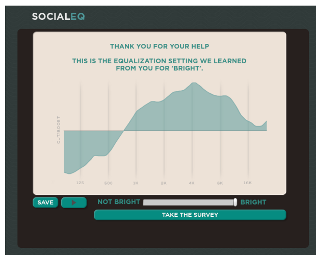
Figure 2. The equalization curve and control slider learned for “bright” in a single session.
